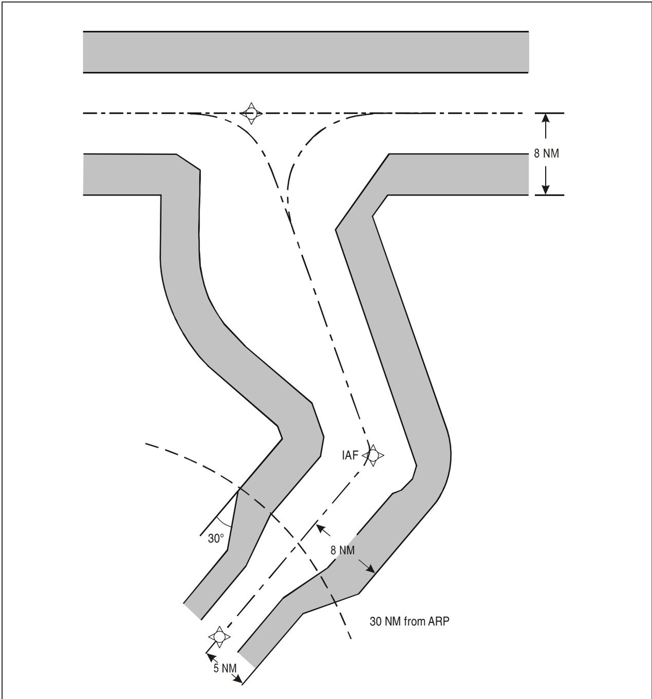
**Figure I-4-2-5. GNSS arrival criteria, IAF beyond 30 NM ARP: 8 NM  $\frac{1}{2}$  AW prior to 30 NM from ARP then 5 NM  $\frac{1}{2}$  AW**
